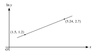
The variables x and y satisfy the equation  $y^2 = Ae^{kx}$ , where A and k are constants. The graph of  $\ln y$  against x is a straight line passing through the points (1.5, 1.2) and (5.24, 2.7) as shown in the diagram.
