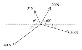
Four coplanar forces act at a point. The magnitudes of the forces are 20 N, 30 N, 40 N and F N. The directions of the forces are as shown in the diagram, where  $\sin \alpha^{\circ} = 0.28$  and  $\sin \beta^{\circ} = 0.6$ .
